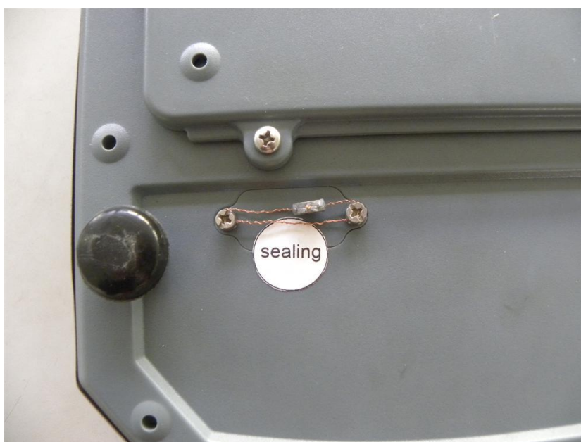
Figure 3 Sealing of scale enclosure with wire and lead or plastic seal in the rod and brittle sticker.
