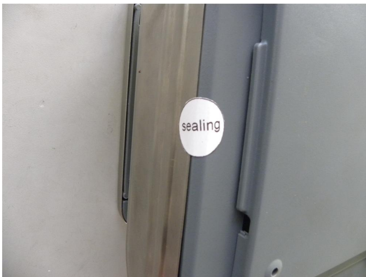
Figure 4 Sealing of scale enclosure with brittle sticker.
